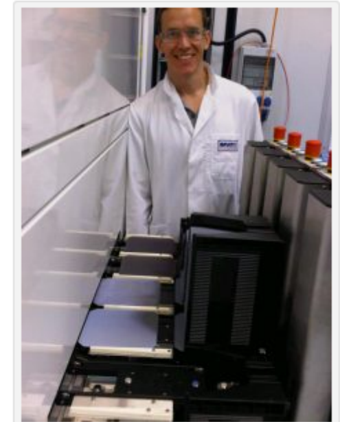
UCF researcher, Kris Davis, stands next to the ACPVD system that deposits metal oxide material onto silicon wafers.
